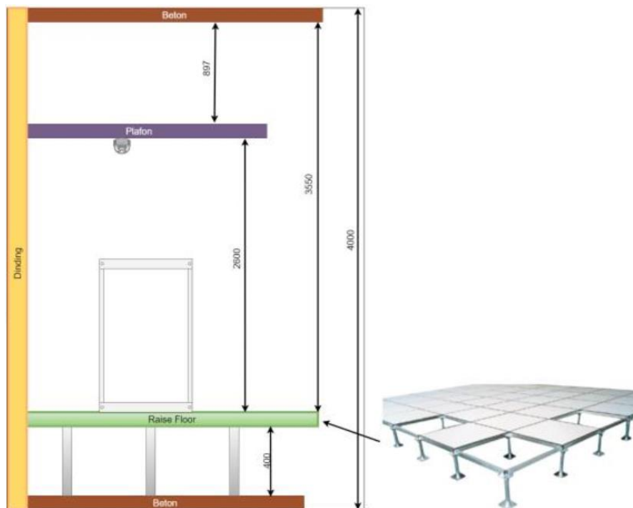
Gambar 40. Layout Raised Access Floor
